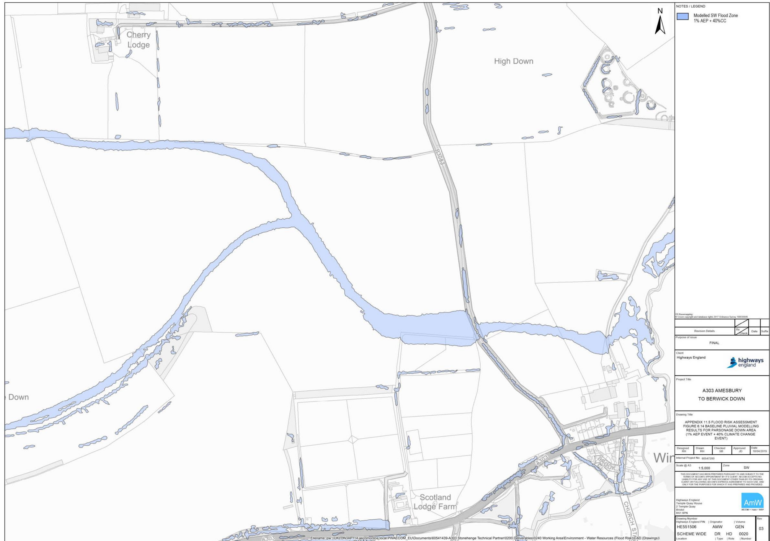
Figure 6.14: Baseline pluvial modelling results for Parsonage Down area (1% AEP + 40% climate change event)
