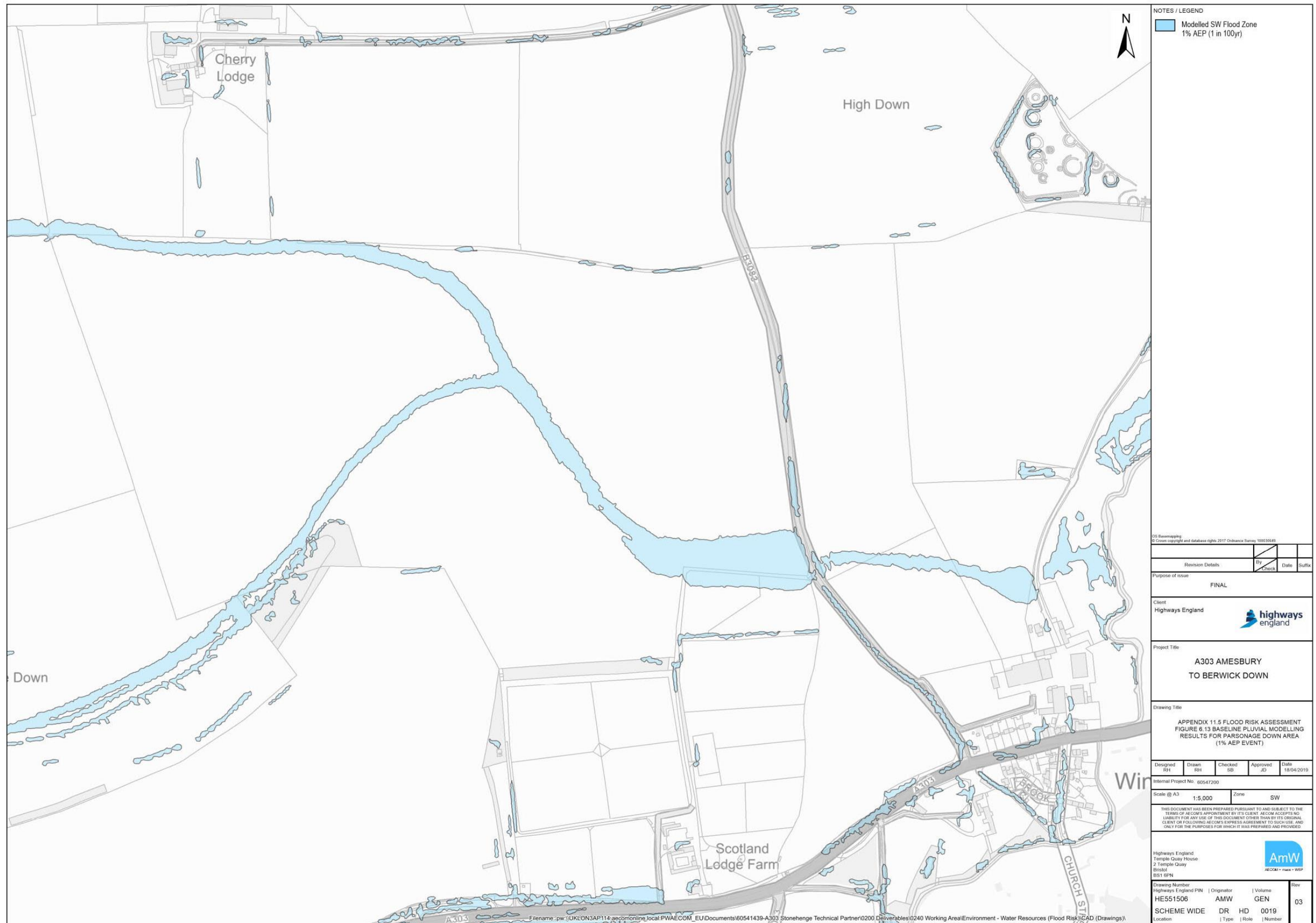
Figure 6.13: Baseline pluvial modelling results for Parsonage Down area (1% AEP event)
