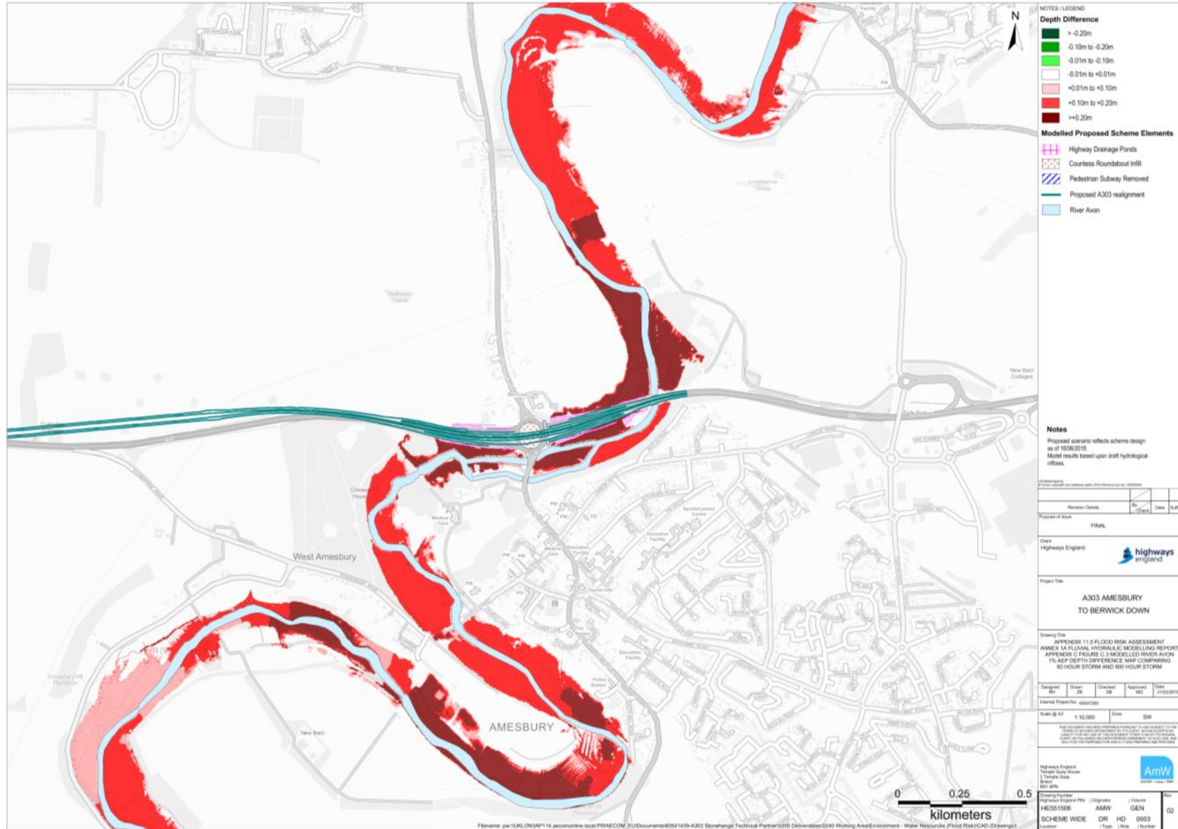
Figure C.3: Depth Difference Map Comparing 1% AEP Event 60 Hour and 800 Hour Storm
