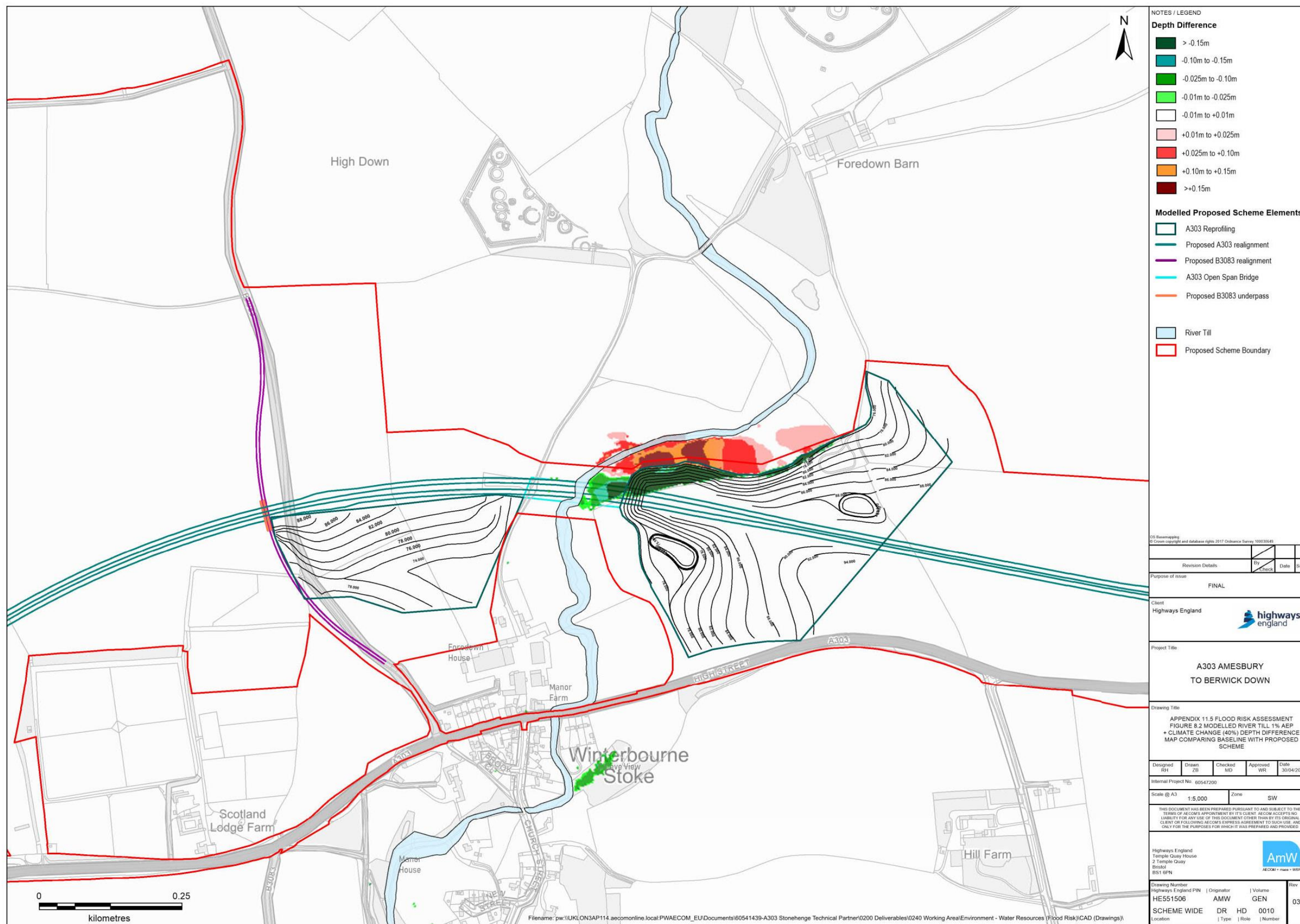
Figure 8.2: Modelled River Till 1% AEP plus Climate Change (+40% Depth Difference Map comparing baseline with proposed scheme
