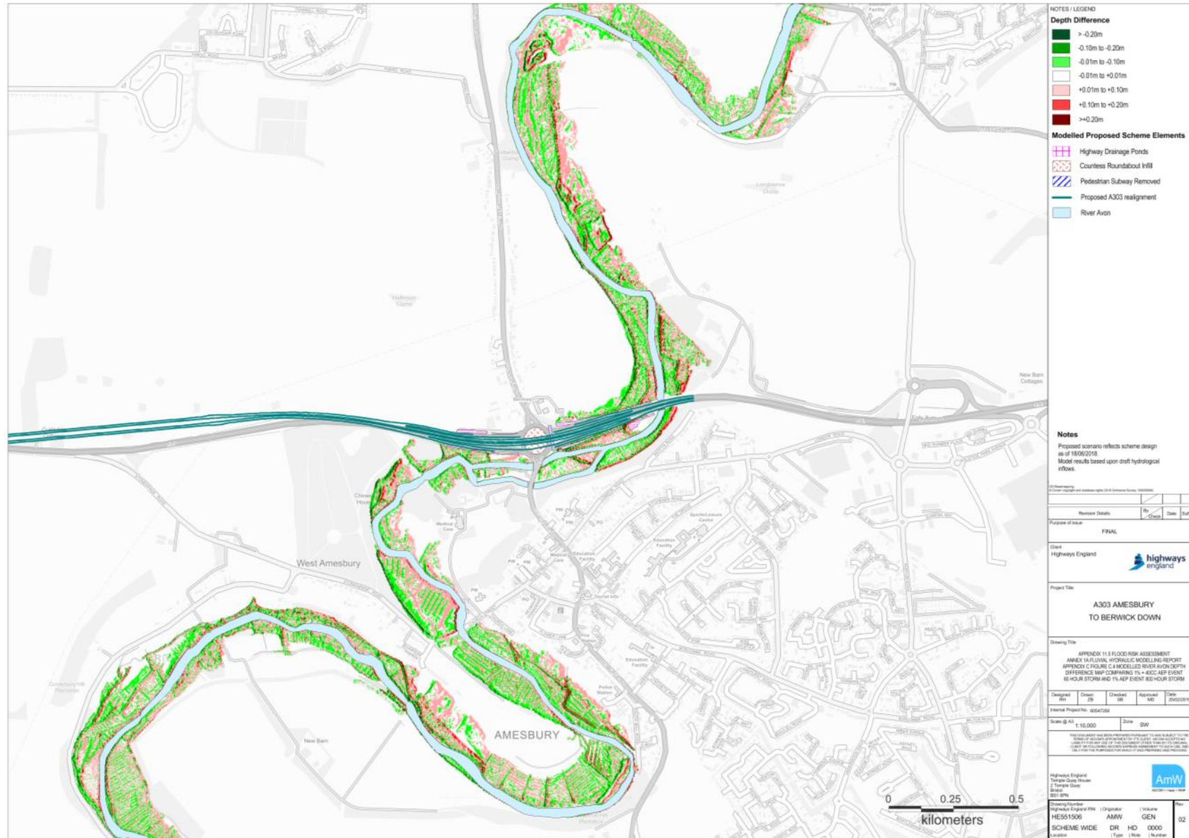
Figure C.4: Depth Difference Map Comparing 1% AEP + 40% Climate Change 60 Hour Storm and 1% AEP 800 Hour Storm
