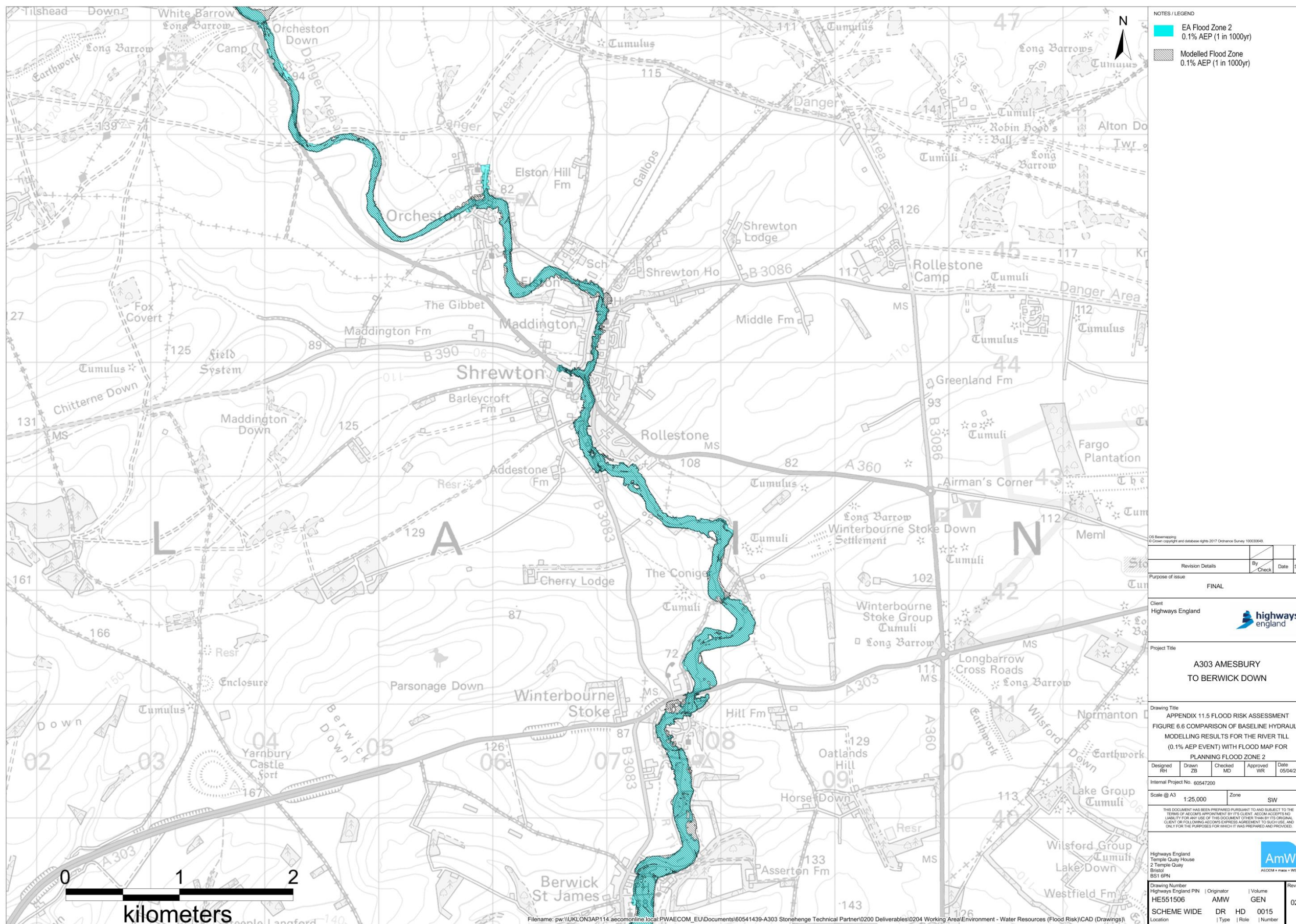
Figure 6.6: Comparison of baseline hydraulic modelling results for River Till (0.1% AEP event) with Flood Map for Planning (Flood Zone 2)
